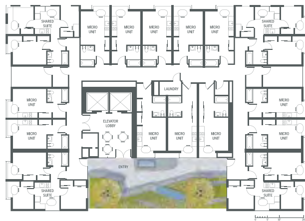
The 12-story building's studios and suites range in size from 274 to 630 square feet. Outdoor living spaces include the courtyard, seen in this plan, and a rooftop garden deck.
