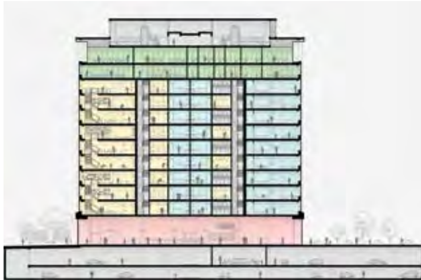
A section view shows an internal staircase (left side) that connects the floors within each of the building's three-story "neighborhoods."
